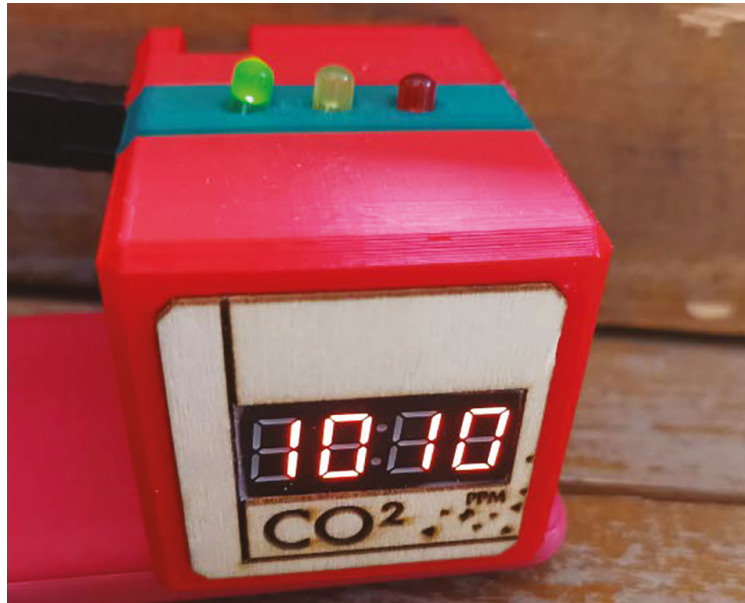
Figure 5.18: Finalised sensor showing CO 2 level. Credit: FAB.
